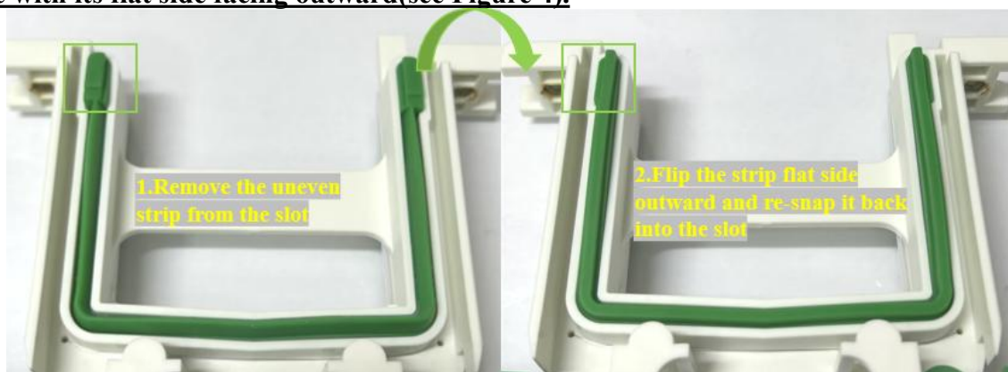
Figure 4: Schematic diagram for replacing the electrophoretic card slot adhesive strip
